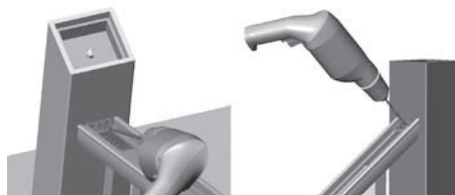
Drawings 20A & 20B: DRILL PILOT HOLES WITH LONG DRILL BIT
