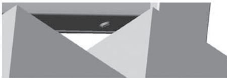
Drawing 17C: UNDERSIDE OF BOTTOM RAIL AFTER SNAPPING RAIL ASSEMBLY INTO PLACE & CLEANING OFF CAULK SQUEEZE-OUT
